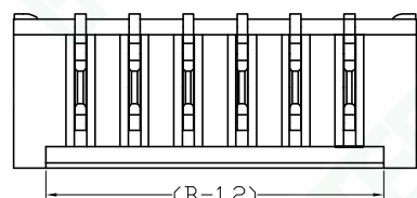
SMT SIDE ENTRY TYPE PCB LAYOUT
